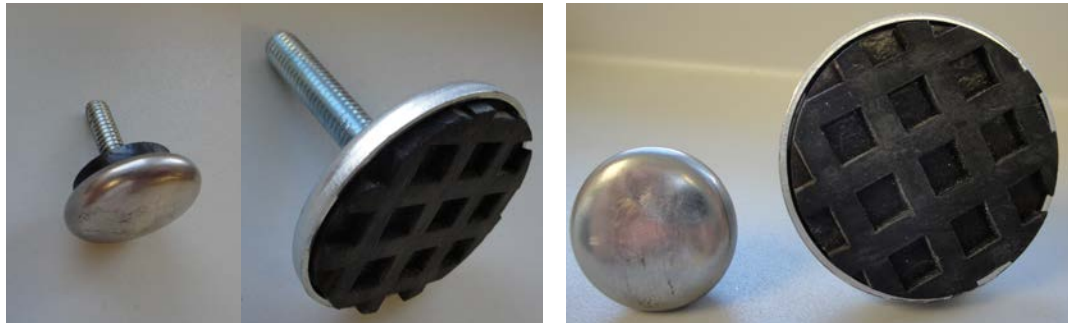
Figure 29: Original smaller feet (2.54 centimeter diameter) with metal bottoms and the new larger feet (5.08 centimeter diameter) with rubber bottoms. The pictures on the left are for composition comparison. The picture on the right is for size comparison.
